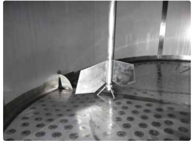
Fig. 5. Agitator in a silo tank with vortex protection.
