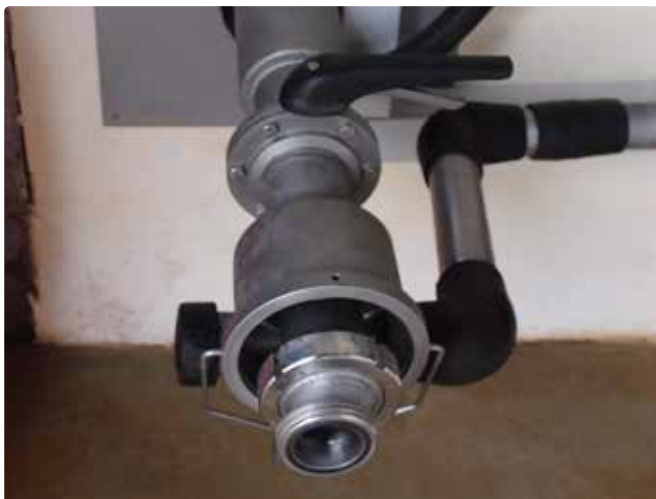
Fig. 6. Example of approved bottom outlet valve.
