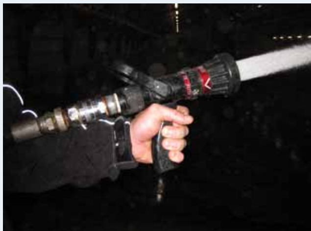
A hose with low pressure and a large amount of water works well for soaking and sluicing.
