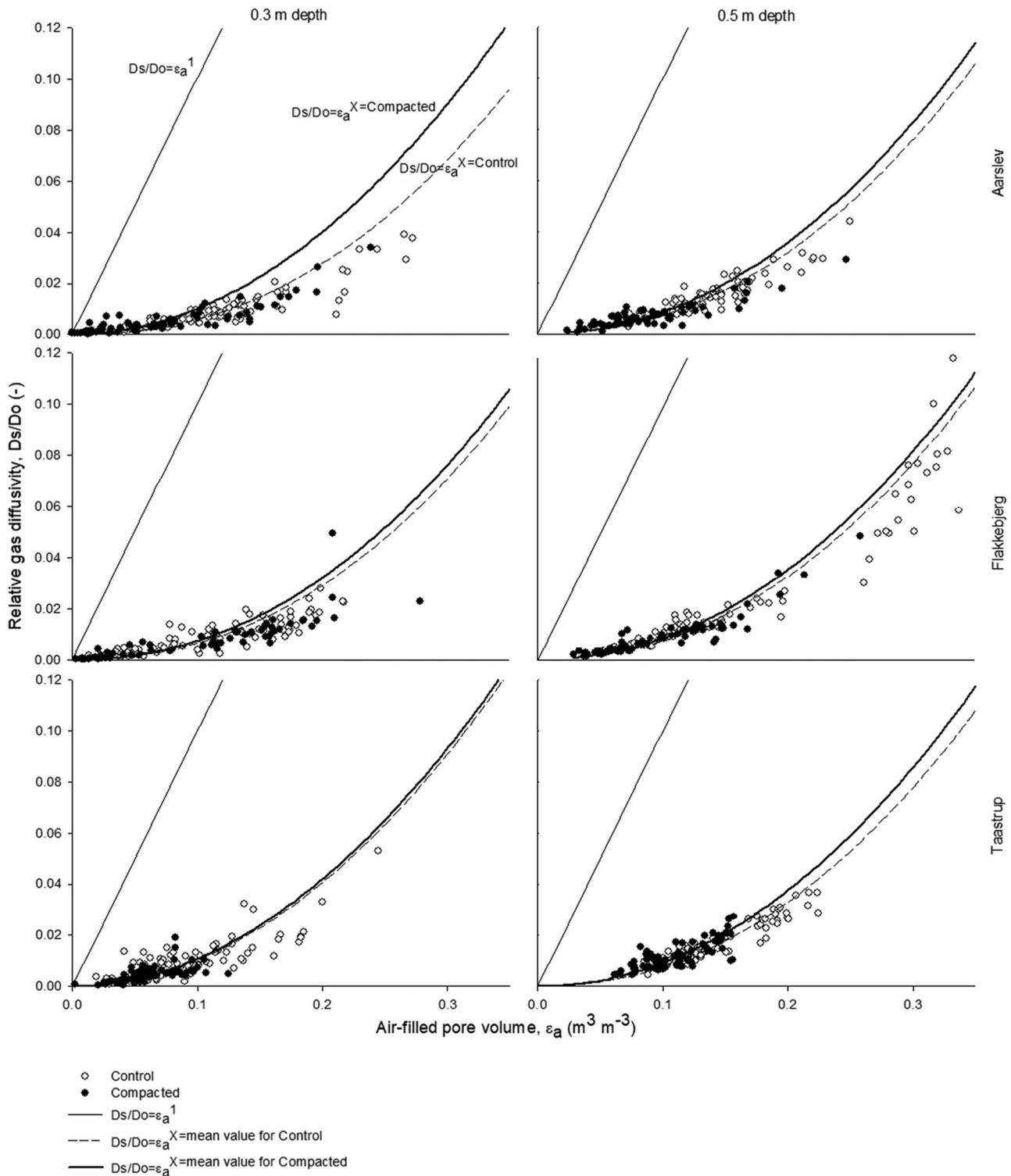
**FIGURE 1** Relative gas diffusivity related to air-filled porosity at  $-100$  hPa matric potential, for three sandy loam soils. Data points fitted by the Buckingham model for  $X = 1$  (fine solid lines) and  $X =$  mean value of  $X$  for the control (dash lines) and for compacted soil (coarse solid lines). Control undergoes no compaction treatment, and compacted soil undergoes heavy traffic with multiple passes (4-5)
