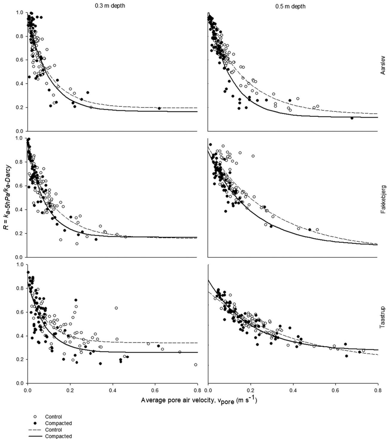
**FIGURE 3** The ratio of non-Darcian and Darcian air permeability ( $R = k_{\alpha-5hPa}/k_{\alpha-Darcy}$ ) to average pore air velocity at  $-100$  hPa matric potential for three sandy loam soils. Control undergoes no compaction treatment, and compacted soil undergoes heavy traffic with multiple passes (4-5)
