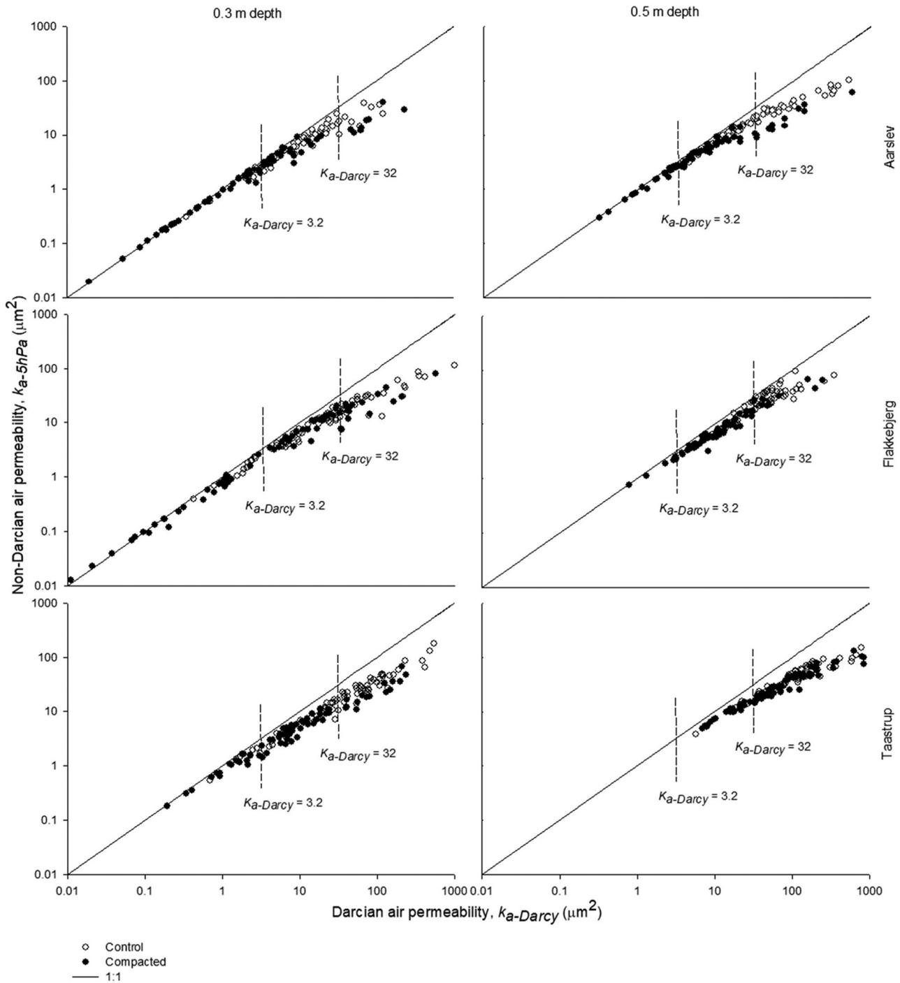
**FIGURE 2** Estimates of the non-Darcian air permeability ( $k_{a-5hPa}$ ) in relation to Darcian air permeability ( $k_{a-Darcy}$ ). Control undergoes no compaction treatment, and compacted soil undergoes heavy traffic with multiple passes (4-5)
