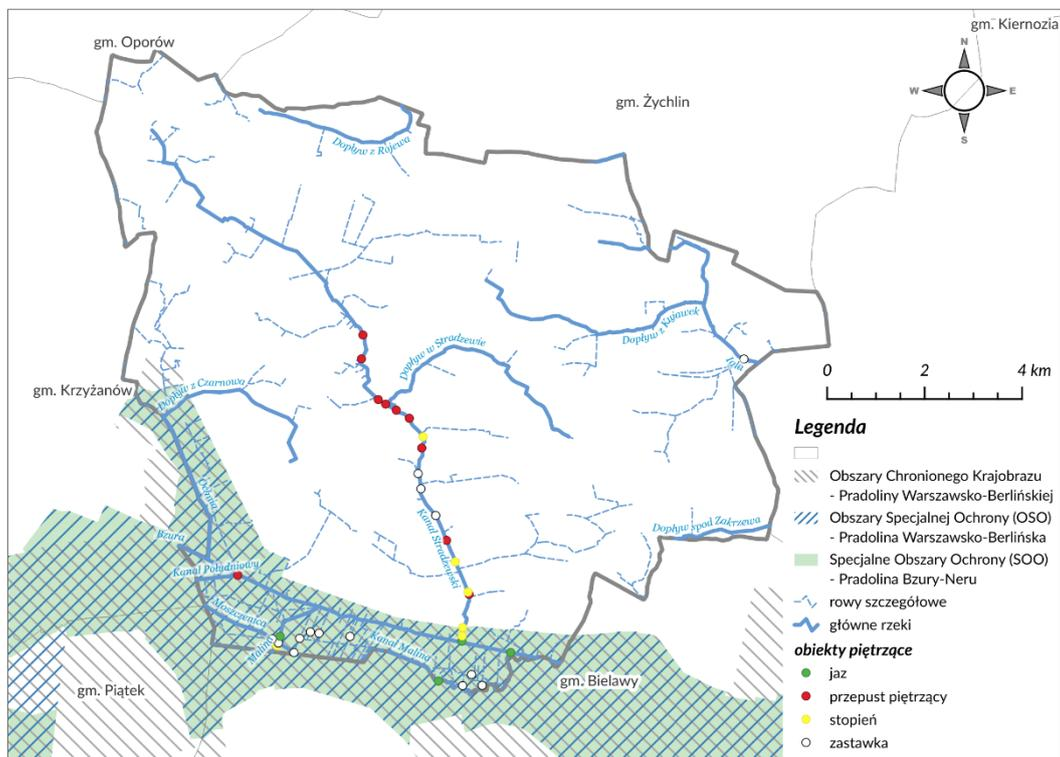
Fig. Hydro-technical facilities in the Stradzewski Channel.
