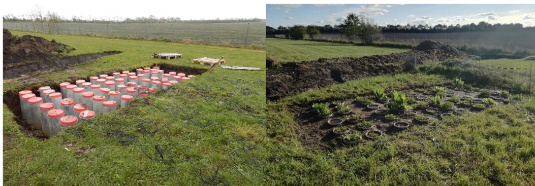
Fig. 1. Installation of the soil samples collected from the Aarslev site at the experimental plot at the Foulum site with the bottom of the samples in contact with the subsoil at 0.50 m depth, and the top level with the soil surface. Samples were installed vertically and surrounded by loose refilled soil.
