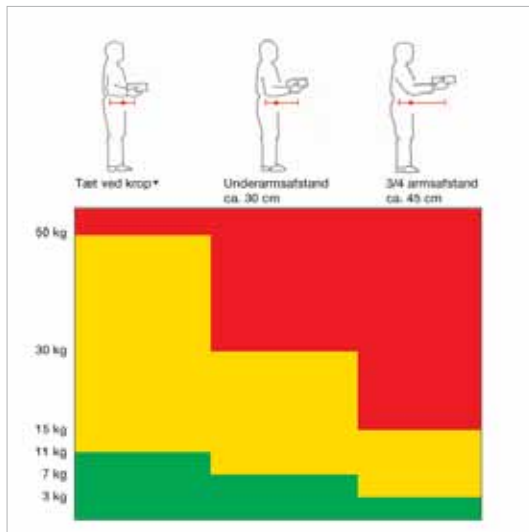
The lifting staircase.
