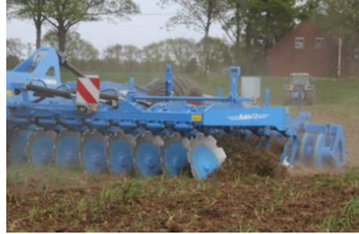
Figur 6.13: Lemken Rubin 12 - aggressive 736 mm tallerkner. Foto: Lemken
